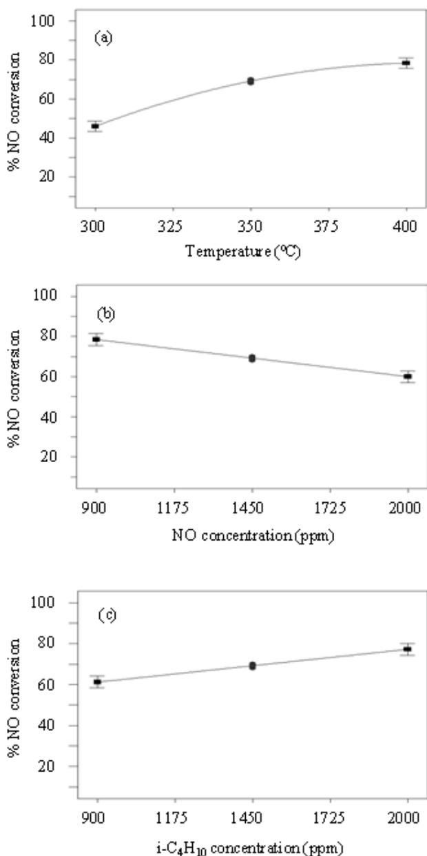
Fig. 2: Influences of (a) reaction temperature (b) NO concentration and (c) iso-butane (i-C<sub>4</sub>H<sub>10</sub>) concentration on the NO conversion (Other variables were set at their respective center points).
