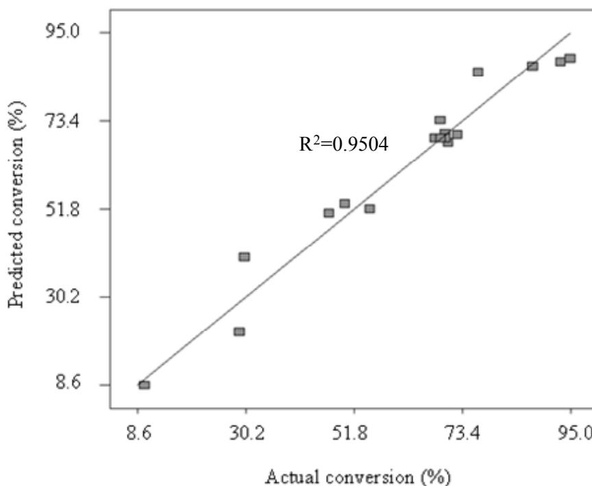
Fig. 1: Parity plot between the predicted and actual data for the NO reduction reaction.
