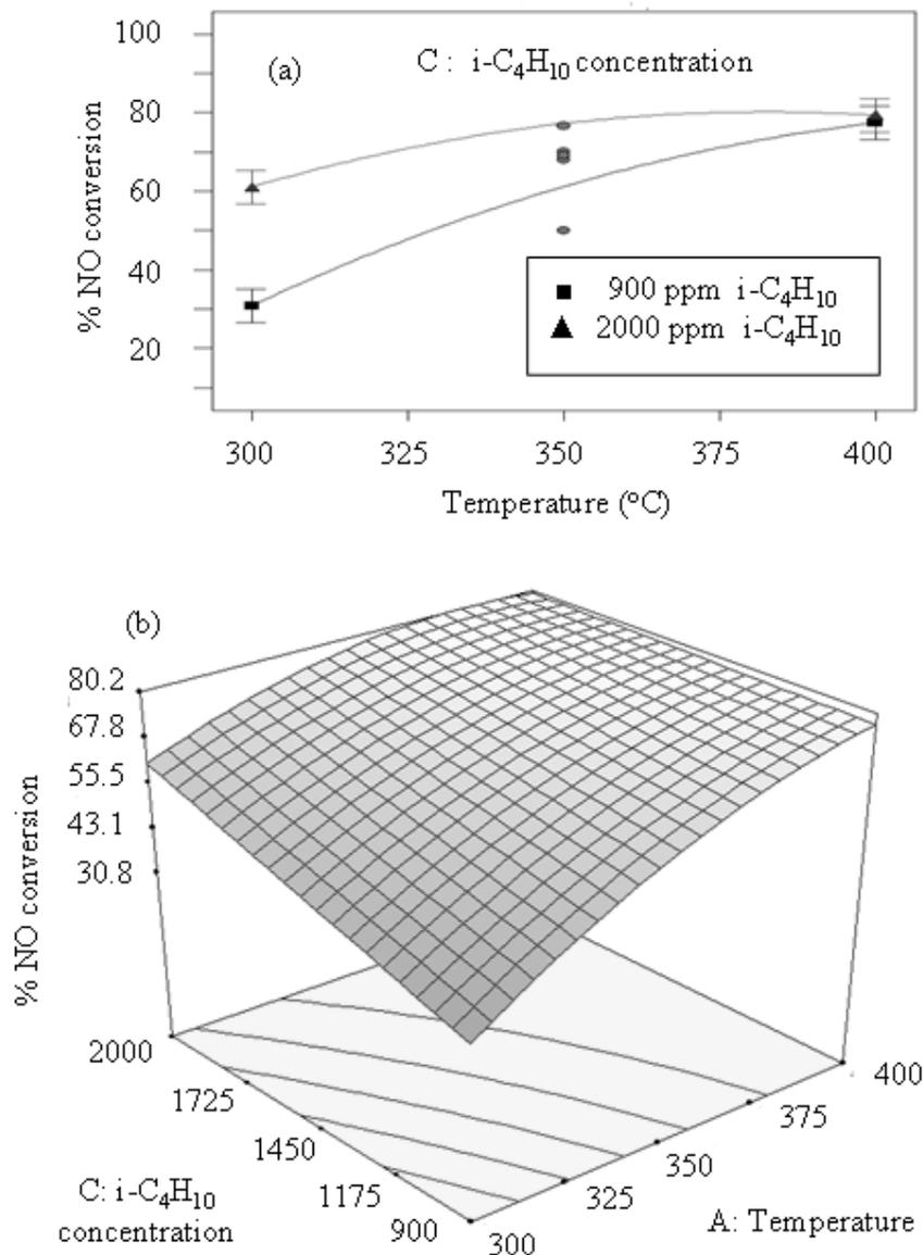
Fig. 3: Effects of iso-butane (i-C<sub>4</sub>H<sub>10</sub>) concentration and temperature on NO conversion shown in an interaction plot
