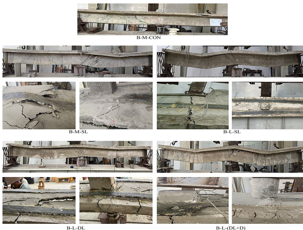
Figure 9. Crack patterns and failure modes of the tested continuous RC beam specimens.
