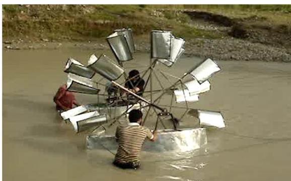
Fig. 4: Battery-based micro-hydropower plant on catamaran for free water flow operation designed and fabricated in GIK Institute of Pakistan.
