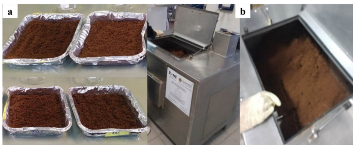
Figure 1. Scale-up procedure of microbial coagulant, a) tray foil, b) rotatory drum bioreactor.
