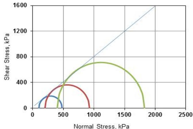
Fig. 14: Mohr circles and the corresponding Mohr envelop.
