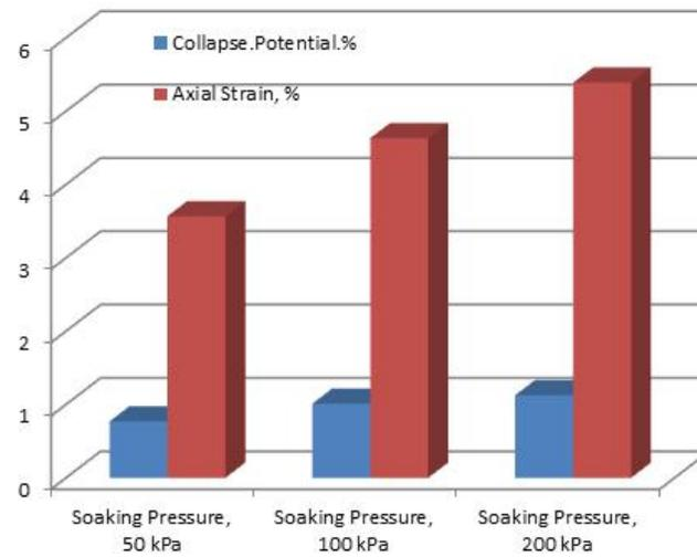
Fig. 7: Collapse Potential (CP) values, the axial strain and soaking pressure.
