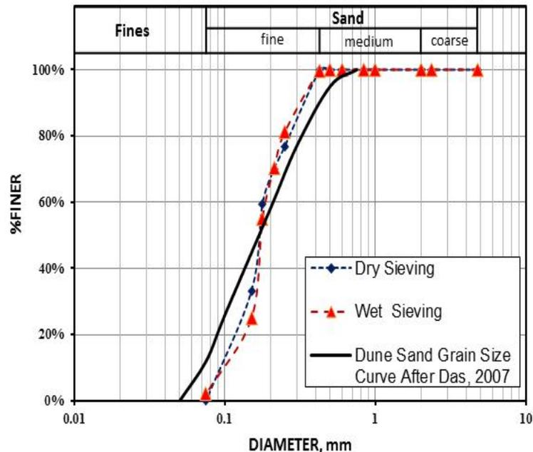
Fig. 3: The particle size distribution curves [9].
