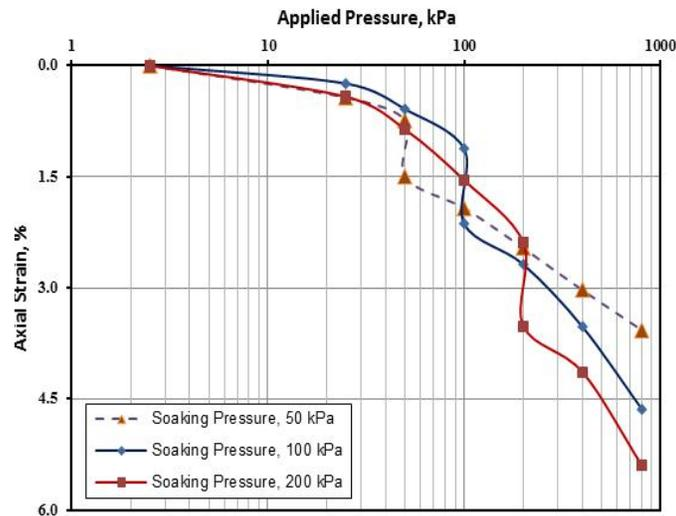
Fig. 6: Single collapse tests results.
