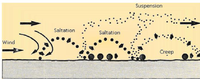
Fig. 2: Methods of grains movement [8].
