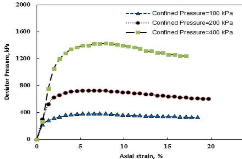
Fig. 13: The principal stress difference versus the axial strain.
