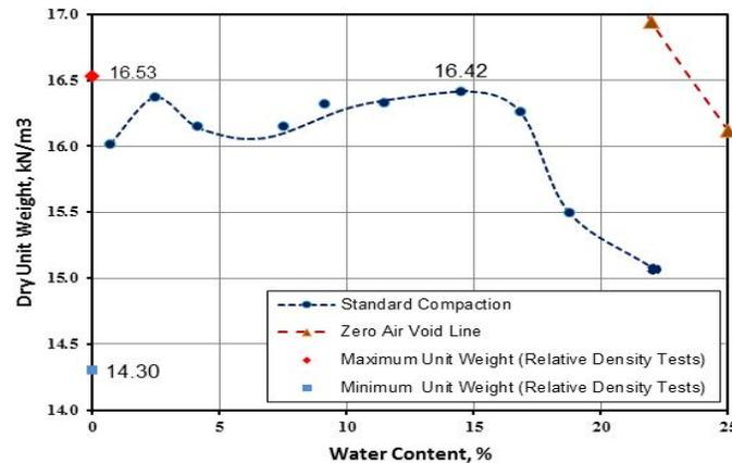
Fig. 4: Compaction and relative density tests results.
