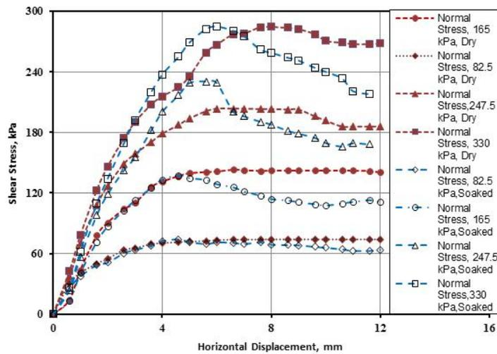
Fig. 10: The stress-strain curves for dry and soaked specimens.
