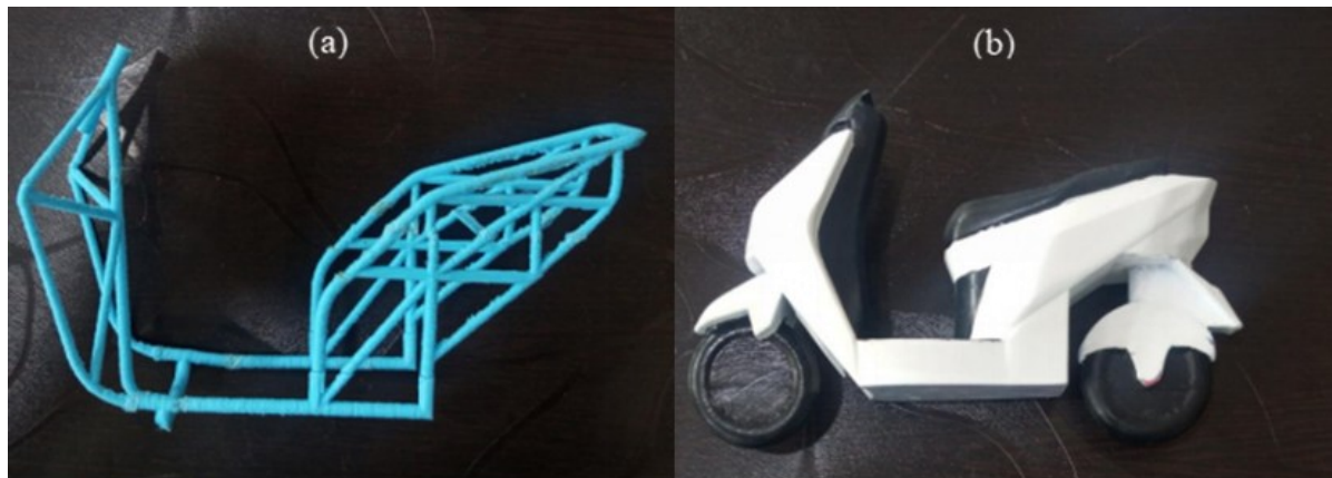
Figure 4. Scaled 3D-printed models of (a) hybrid trellis chassis and (b) complete scooter with a body shell.
