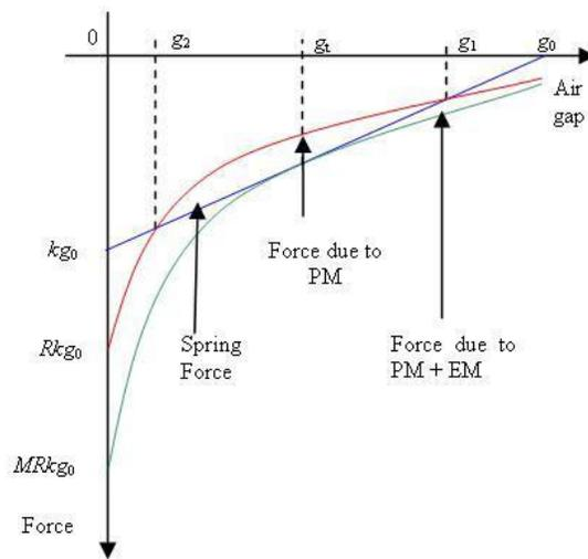
Fig. 5: Relative position of force characteristics.
