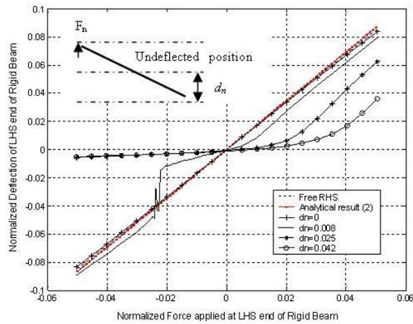
Fig. 9: Force – deflection characteristics of the LHS end when RHS end is pressed down against a dead stop distance  $d$  below the undeformed position of rigid beam.
