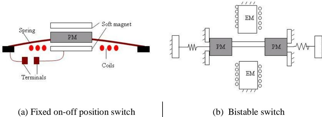
Fig. 7: Schematic designs of bistable, latching, electromagnetic switch.
