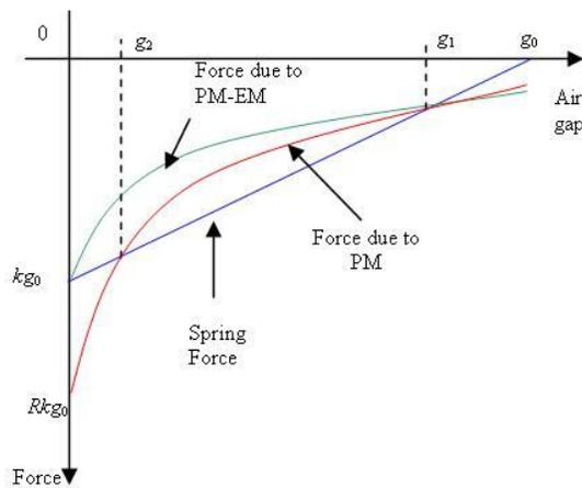
Fig. 6: Relative position of force characteristics of microrelay on the verge of latching of microrelay on the verge on unlatching.
