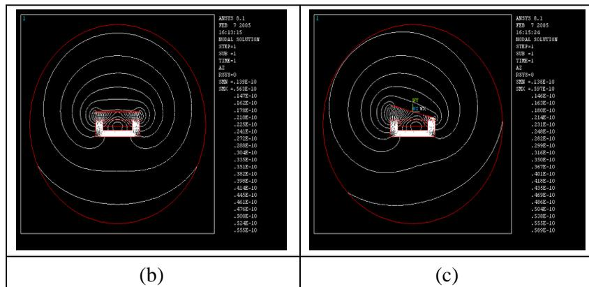
Fig. 10: FEA of magnetic circuit and the magnetic flux patterns for horizontal and tilted position
