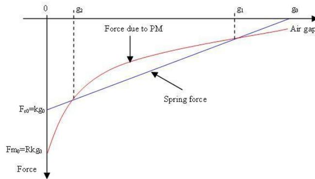
Fig. 4: Spring and Magnetic Forces as functions of air gap.
