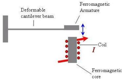
Fig. 2: Magnetization-type actuator.
