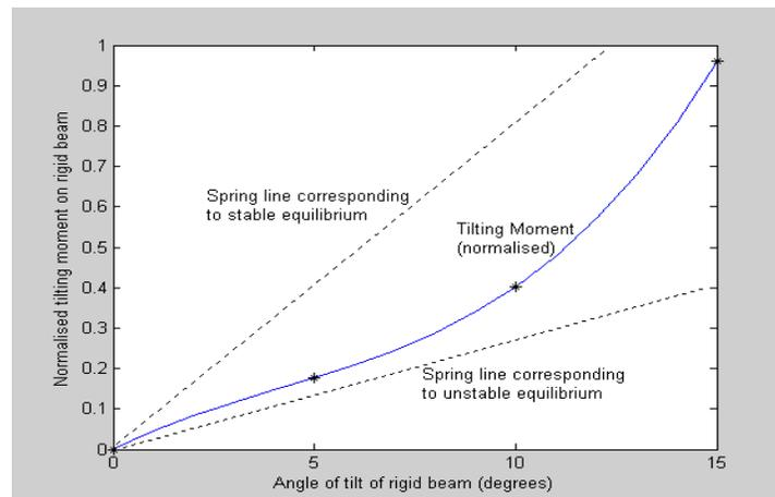
Fig. 11: Tilting moment at different angle
