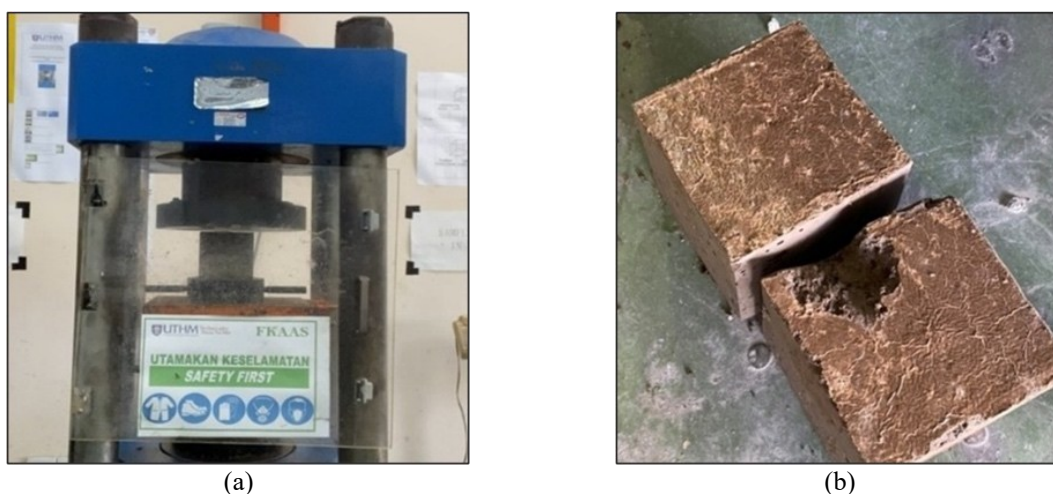
Figure 4. (a) Compressive strength test and (b) Concrete cube of S/S matrices samples
