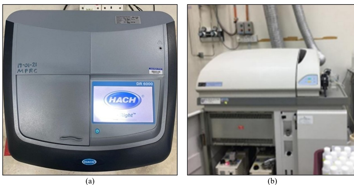
Figure 6. (a) HACH DR600 equipment and (b) Inductively Coupled Plasma Mass Spectroscopy (ICP-MS)
