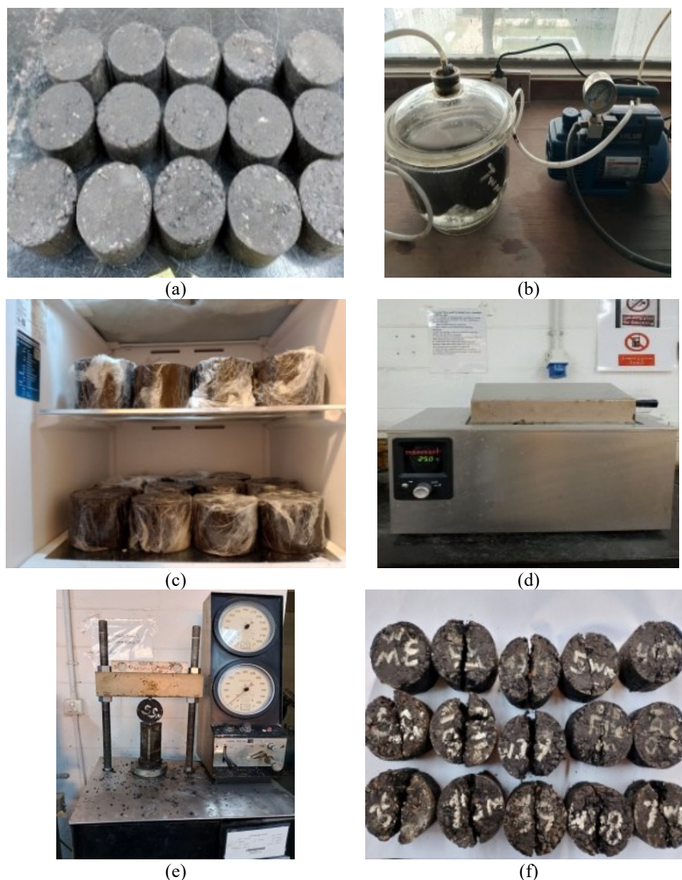
Figure 5. Stages of water damage test: (a) samples before test; (b) saturation process; (c) freezing cycle; (d) thawing cycle; (e) sample testing; and (f) fractured samples.
