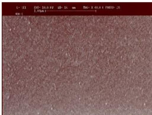
Fig. 1: SEM micrographs of the surface of the sintered alumina membrane (sintered at 400°C) with with  $\times 500$  magnification
