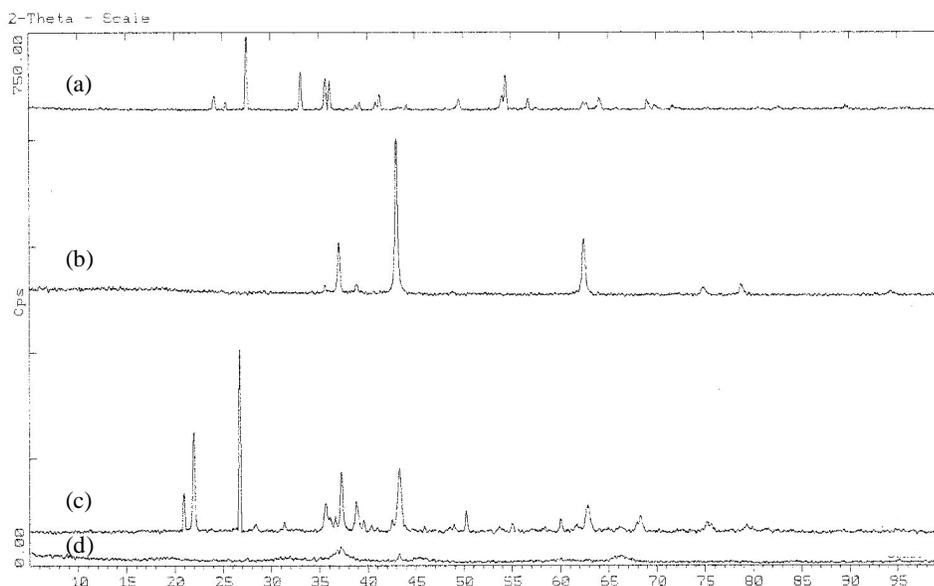
Fig. 2: The XRD pattern of the fresh catalyst containing Cu/Ni supported on (a) TiO<sub>2</sub>, (b) MgO, (c) SiO<sub>2</sub>, and (d) Al<sub>2</sub>O<sub>3</sub>.
