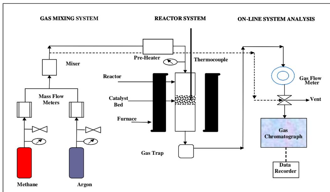
Fig. 1: Schematic diagram of the reactor system.
