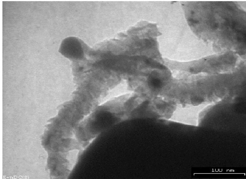
Fig. 5: The transmission electron microscope image of the nanotube produced on Cu/Ni supported on SiO<sub>2</sub> at 998 K and GHSV of 2700 h<sup>-1</sup>.
