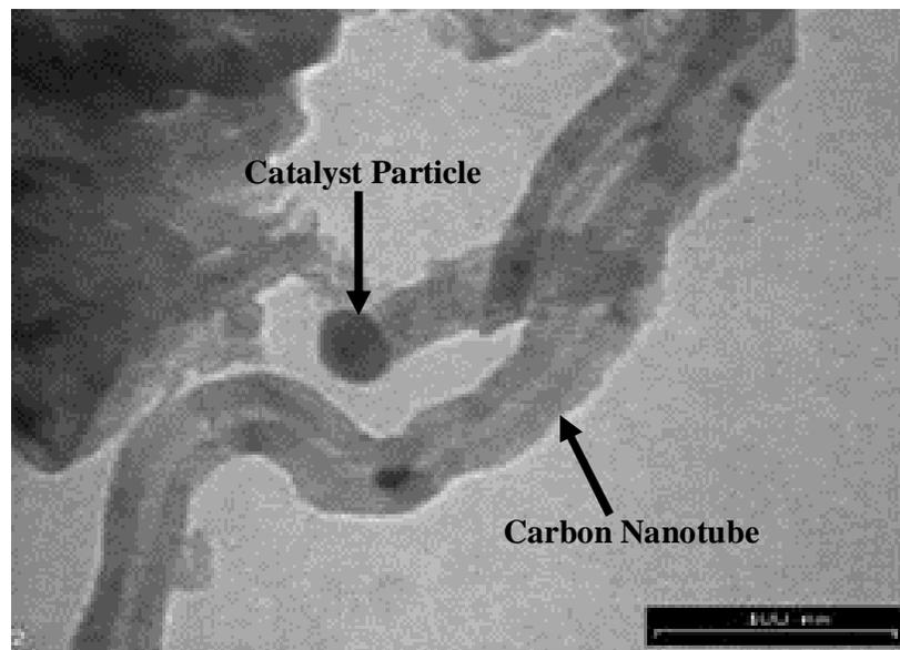
Fig. 6: The transmission electron microscope image of the nanotube produced on Cu/Ni supported on TiO<sub>2</sub> at 998 K and GHSV of 2700 h<sup>-1</sup>.
