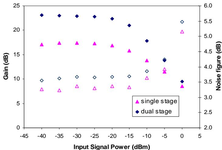
Fig. 4: Gain (closed) and noise figure (clear) as a function of input signal power.
