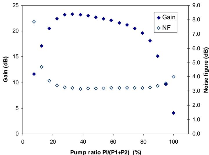
Fig. 3: Gain (closed) and noise figure (clear) as a function of power ratio of pump 1.
