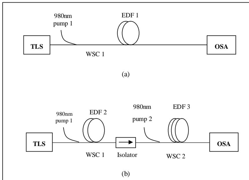
Fig. 1: Configuration of the L-band EDFA (a) single stage (b) dual stage
