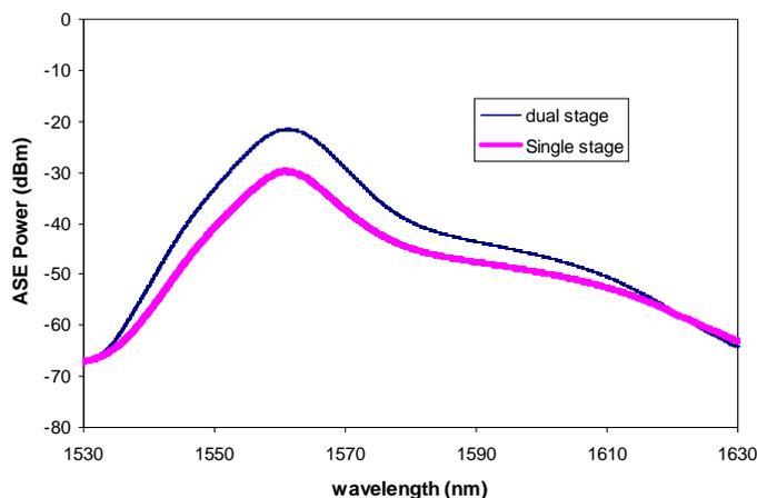
Fig. 2: ASE spectra of the L-band EDFA while the total pump power is fixed at 92mW. For dual stage amplifier, pump 1 and pump 2 are fixed at 35mW and 57mW, respectively.
