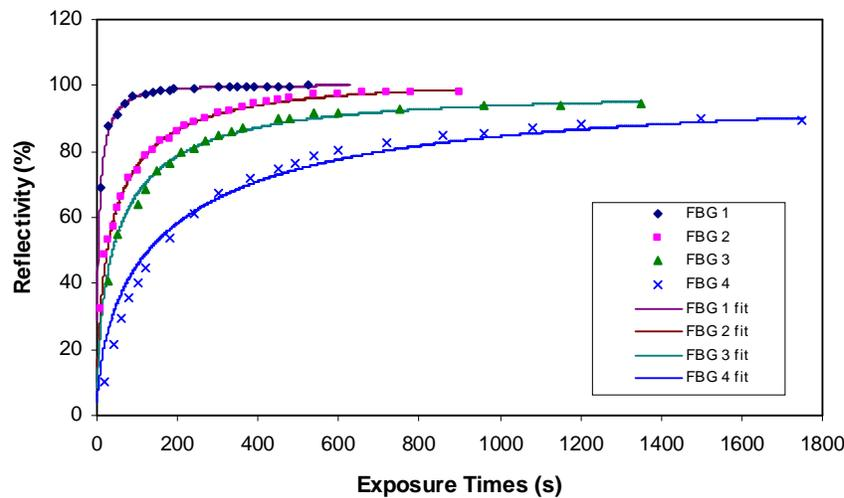
Fig. 1: The FBGs reflectivity as a function of exposure time. The reflectivity growth with time is fit using equation (2), which is explained in the text.
