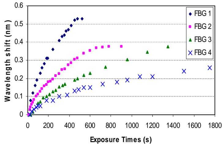
Fig. 2: Bragg wavelength shift with time. There are many factors influencing the wavelength shift and therefore was not fit with theoretical calculation.
