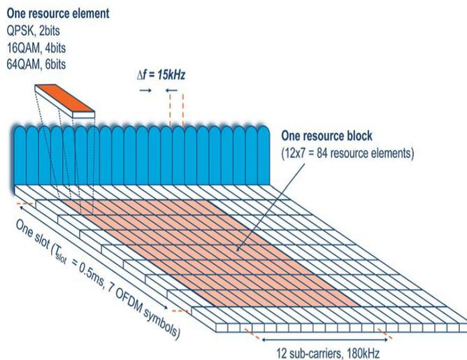
Fig. 1: LTE downlink physical resource based on OFDM [5].
