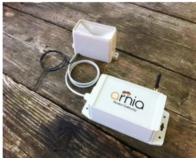
Figure 7. Arnia remote hive monitoring system [10].
