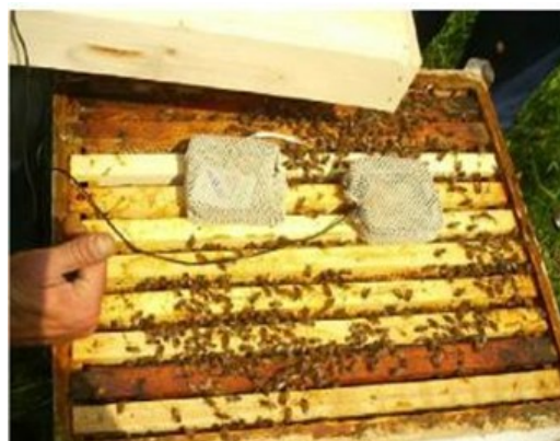
Figure 4. The microphone and Hobo placement inside the beehives [9].
