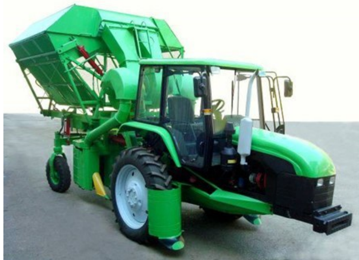
Figure 1. Vertical spindle Cotton Picker.
