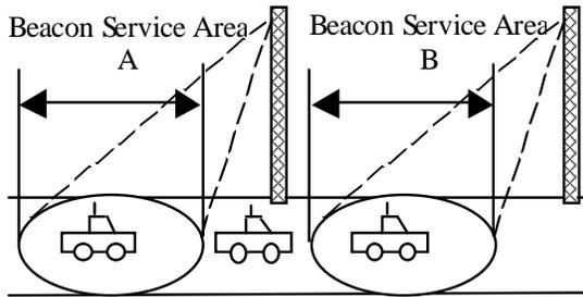
Fig. 1: Vehicular location fixing with proximity devices.
