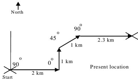
Fig. 2: Vehicular location fixing with dead reckoning.
