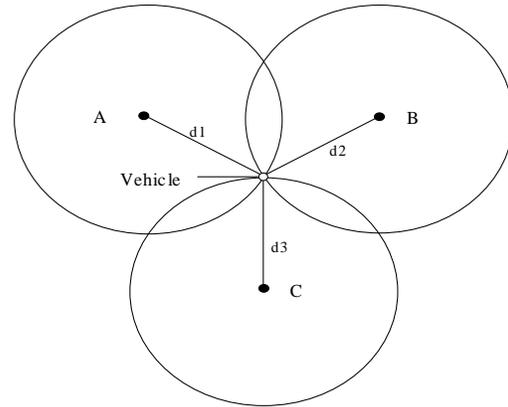
Fig. 3: Vehicular location fixing with trilateration technique.
