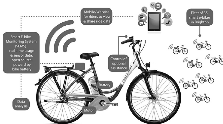
Figure 2. SEMS was developed to collect real-time usage and sensor data, combining open-source software and open hardware (Kiefer & Behrendt, 2016) [15]
