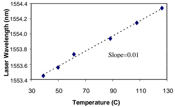
Fig. 4 Fiber laser wavelength against applied temperature
