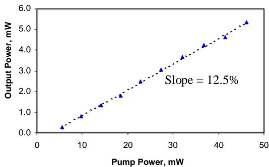
Fig. 2 Output power as a function of coupled in pump power
