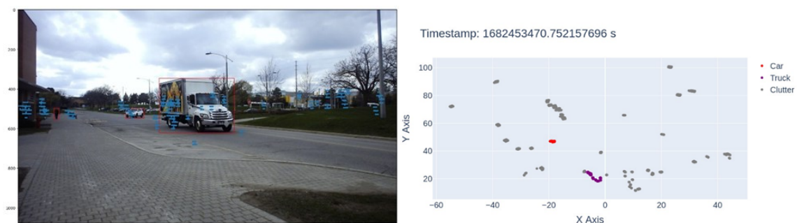
Figure 12. Truck in scene 1. (left) 3D Point cloud projection onto the 2D image. (right) X-Y axis scatter plot for point cloud dataset with target class.
