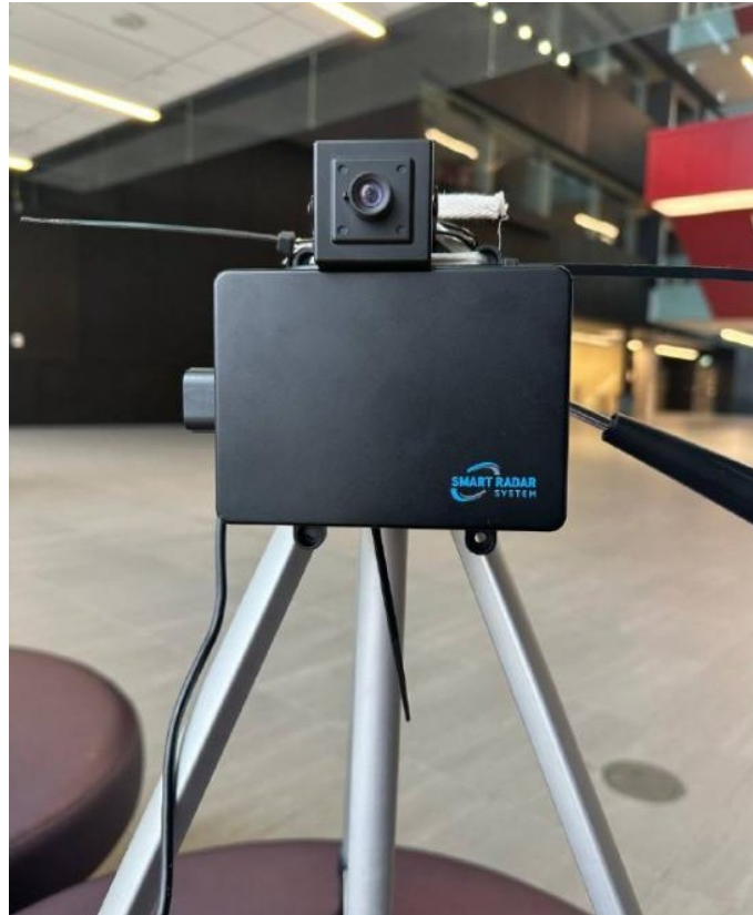
Figure 2. Camera and radar sensors setup.
