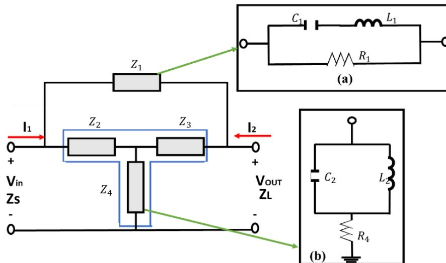
Figure 1. The proposed single bridged- T pre-equalizer circuit.
