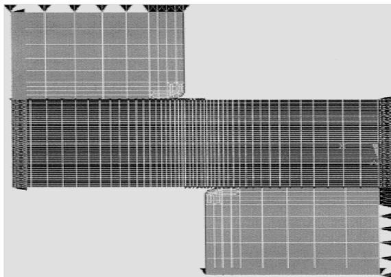
Fig. 2: Mesh in the shearing zone.
