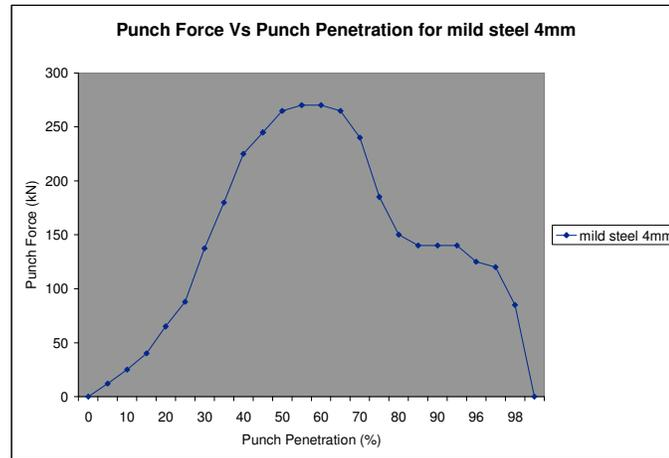
Fig. 6: Punch force vs punch penetration of blanking process (4 mm MS sheet).
