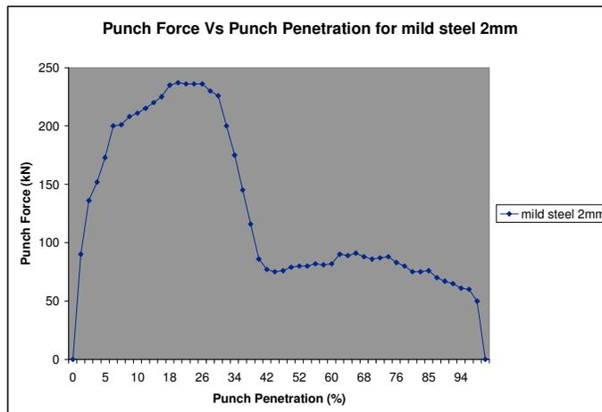
Fig. 5: Punch force vs punch penetration of blanking process (2 mm MS sheet).
