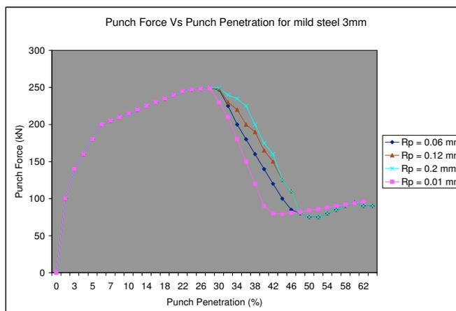
Fig. 9: Simulation of punch force against punch penetration for various punch edge radius for blanking of 3 mm MS sheet.
