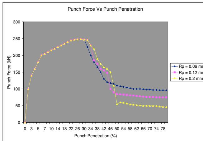
Fig. 8: Experimental results for punch force vs punch penetration of 3 mm MS Sheet for various punch edge radii reported by Hambli and Potiron [12].
