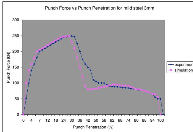
Fig. 7: Simulation compared with experimental results of Hambli and Potiron [12].
