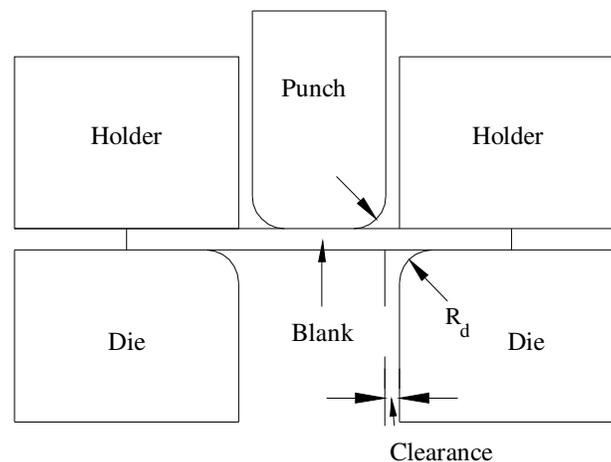
Fig. 1: Geometry of punch, die, blank holder, sheet and clearance.
