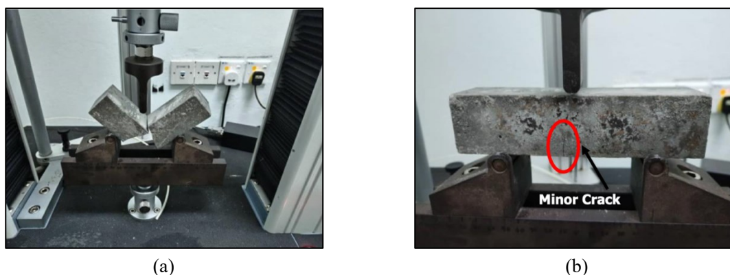
Fig. 11: The conditions of the (a) control and (b) AC-CF specimens after failure.
