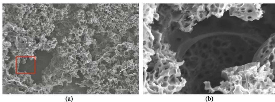
Fig. 2: SEM images of produced BF-AC magnification of (a) x1000, (b) x2500.
