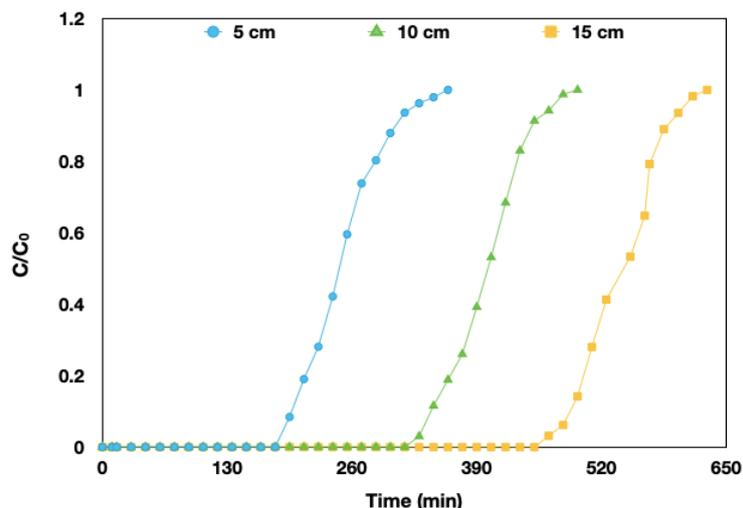
Fig. 6: Phenol adsorption breakthrough curves at various bed heights (5, 10 and 15 cm), 20 mL/min flowrate, and 150 mg/L initial phenol concentration.
