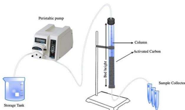
Fig. 1: Bed column experimental setup.
