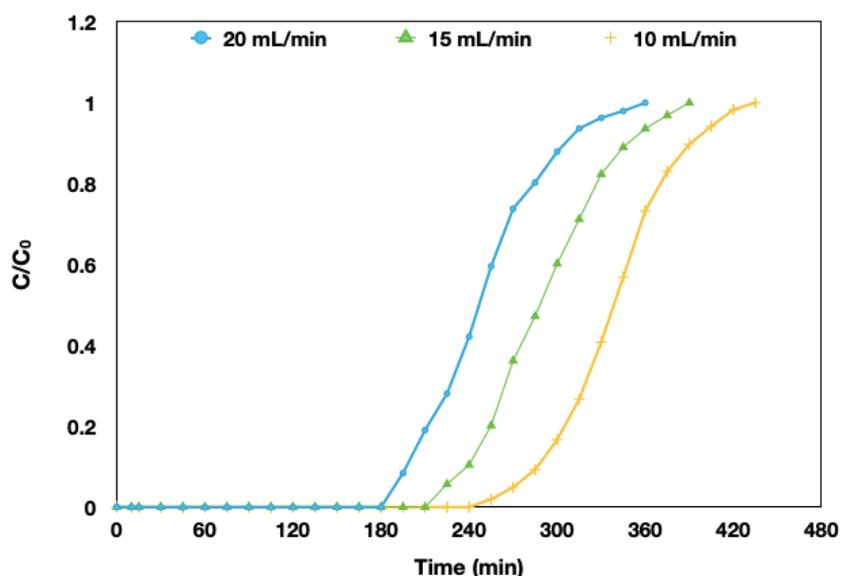
Fig. 5: Phenol adsorption breakthrough curves at various flowrates (10,15 and 20 mL/min), 5 cm bed height, and 150 mg/L initial phenol concentration.
