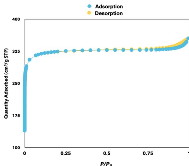
Fig. 4: N<sub>2</sub> adsorption–desorption isotherms of produced BF-AC.
