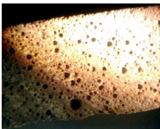
Fig. 1: The effect of lithium carbonate content on the developed ceramic's porosity.
