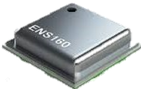
Fig. 1: ENS 160 Gas Sensor, Sciosense B.V., Eindhoven, Netherlands [33]
