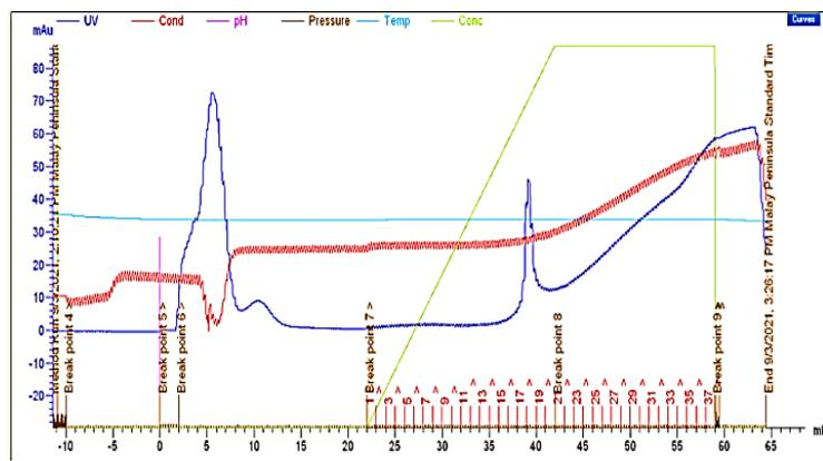
Fig. 4: Chromatogram of the purified samples from affinity chromatography of 2 mL loading volume of recombinant collagen-like protein lysates on Ni-Sepharose resin. Binding buffer contain 20 mM of  $\text{Na}_2\text{HPO}_4$ , 0.5M NaCl at pH 7.4. Elution buffer contained 20 mM  $\text{Na}_2\text{HPO}_4$ , 0.5 M NaCl and 0.5 M imidazole, at pH 7.4. Fractions (1 mL/tube) were collected at flow rate of 1 mL/min.
