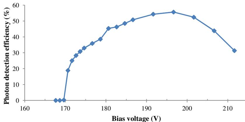
Fig. 5: Photon detection efficiency vs. bias voltage.
