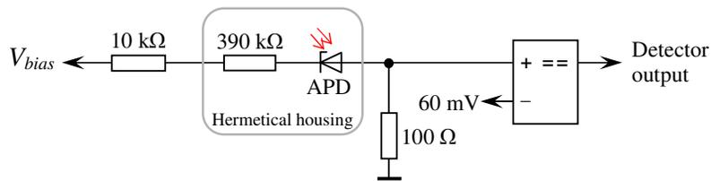
Fig. 1: Passively-quenched detector circuit.
