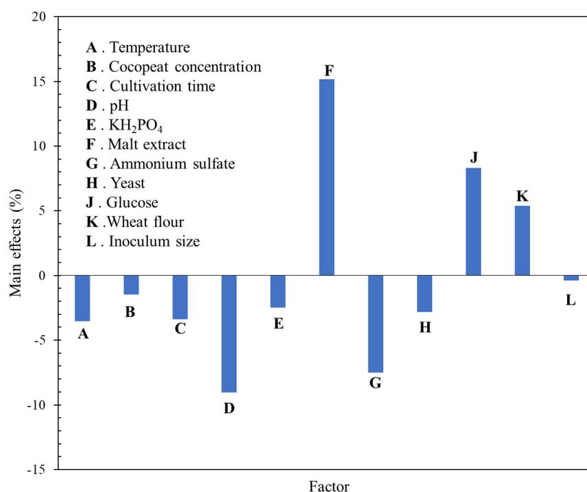
Fig. 5. Main effects of the nutritional components on Flocculation activity
