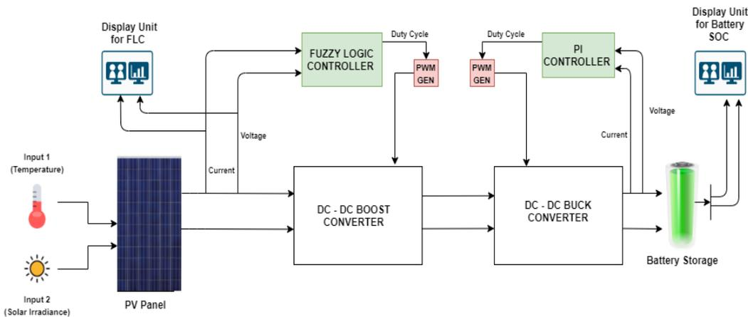
Fig. 3: Proposed system for MPPT and battery charge control of the PV panel.
