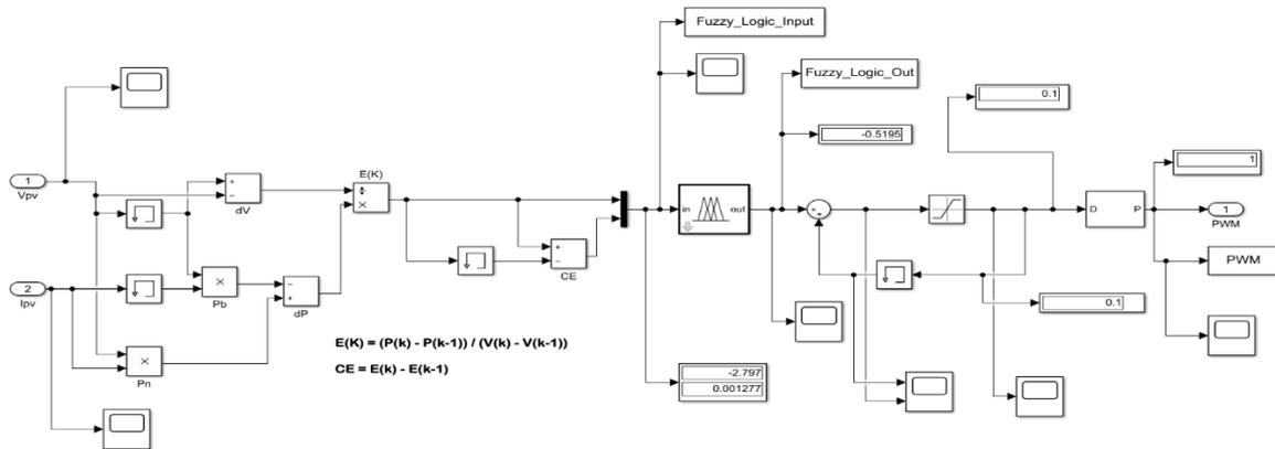
Fig. 7: The MPPT algorithm for the FLC.
