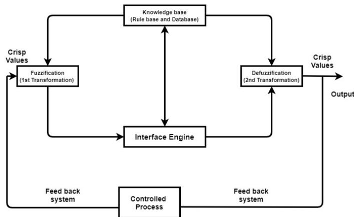
Fig. 1: Block diagram for FLC.
