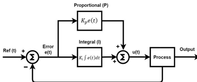
Fig. 2: PI controller block diagram.
