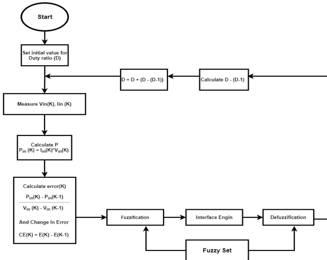
Fig. 6: The operational flow chart of the FLC.
