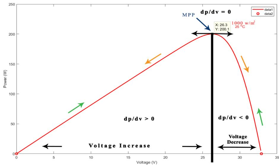
Fig. 5: Power vs voltage characteristic for MPPT algorithm.
