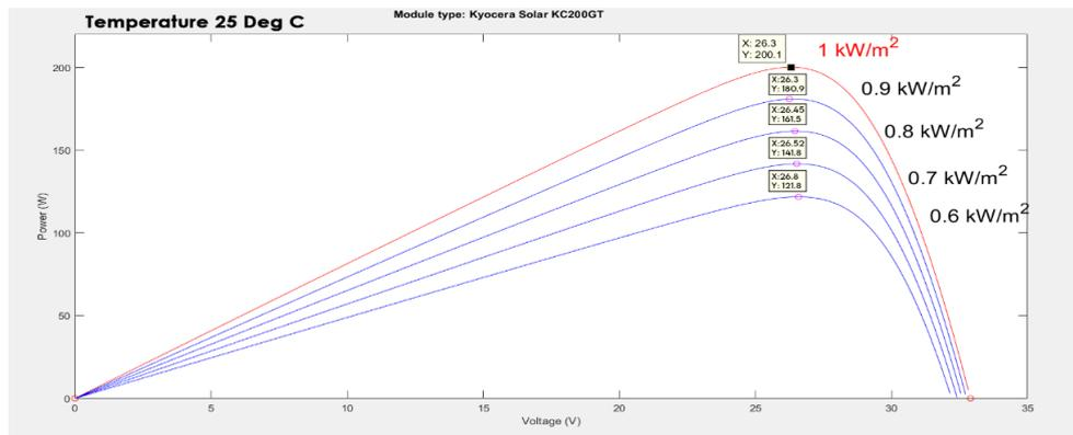
Fig. 11: P-V characteristic curve under variable solar irradiance.
