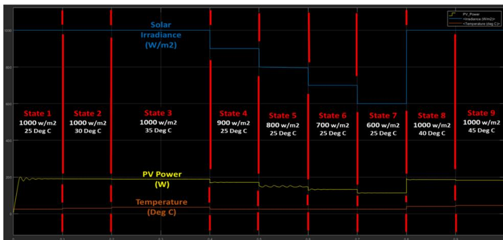
Fig. 13: PV power graph in terms of variable inputs.
