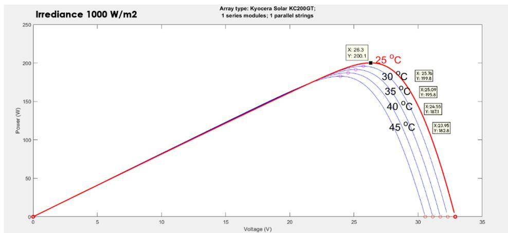
Fig. 12: P-V characteristic curve under variable temperature.
