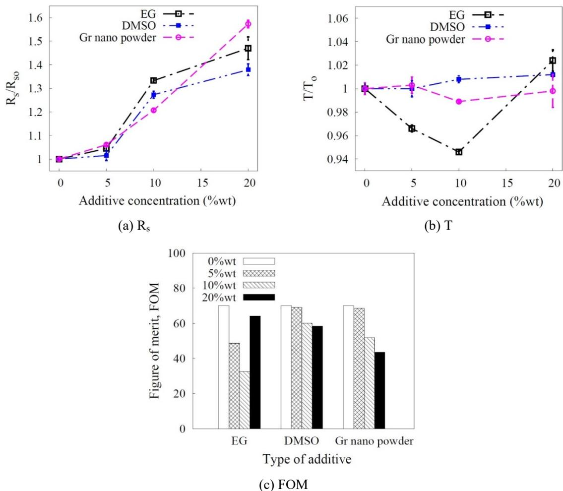
Fig. 9: Effect of adding different concentration of different type additives (EG, DMSO, Gr nano powder) towards the changes of (a)  $R_s$ , (b)  $T$  and (c) FOM of PEDOT:PSS transparent conductive thin film.
