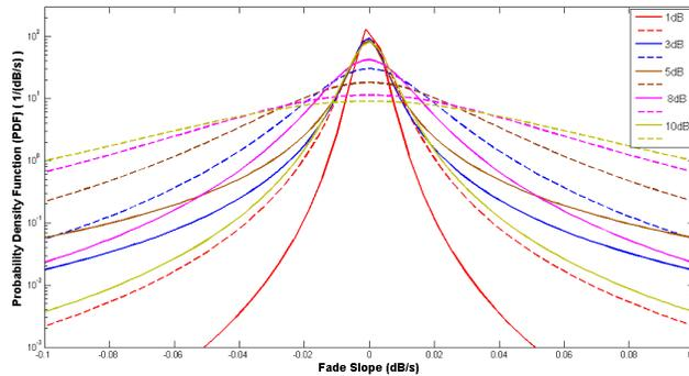
Fig. 4: PDF comparison between fitting of measured data (solid line) and ITU-R (dash line) model for 1s sampling time.
