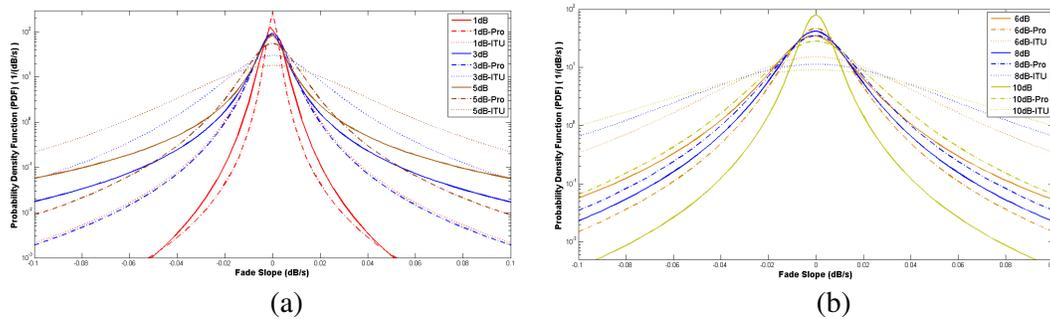
Fig. 6: PDF comparison among Measurement and model with different values of  $s$ -parameters of (a) 1dB to 5dB attenuations and (b) 6dB to 10dB attenuations levels.
