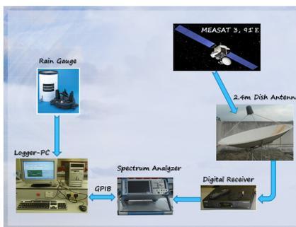
Fig. 1: Experimental setup for measurement at Ku-band signal over earth-space path at Satellite Communications Lab, IIUM.
