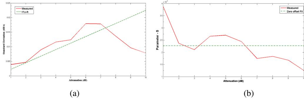
Fig. 5: (a) Comparison of standard deviations between measured data (solid line) and predicted by ITU-R prediction models (dash line), (b) The measured value of  $S$  as a function of attenuations between measurement (solid line) and Zero Offset fit (ZOF) (dash line).
