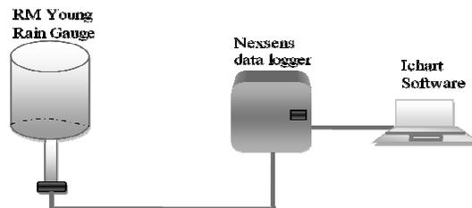
Fig. 1: Rain gauge and data logger block diagram.
