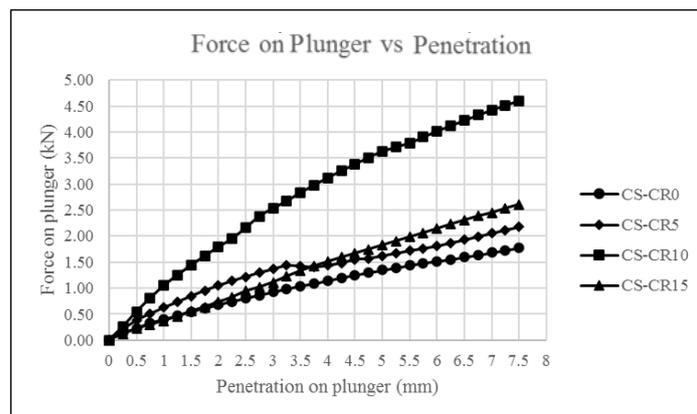
Fig. 7: California Bearing Ratio result.
