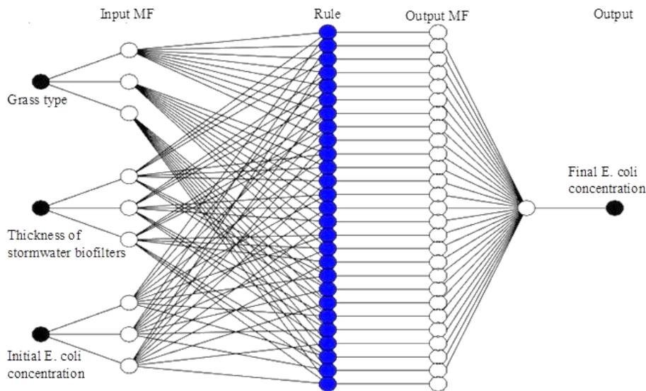
Fig. 5: The architecture of the ANFIS model.
