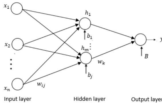
Fig. 2. The general architecture of the FBNN model.
