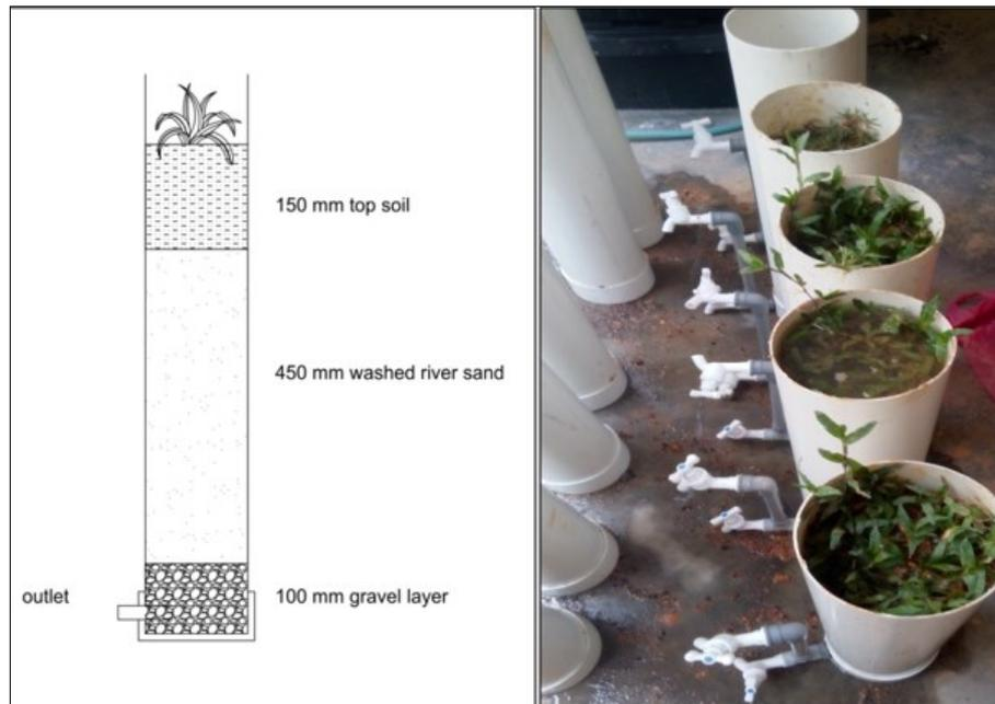
Fig. 1: The setup of biofilter columns used in this study.
