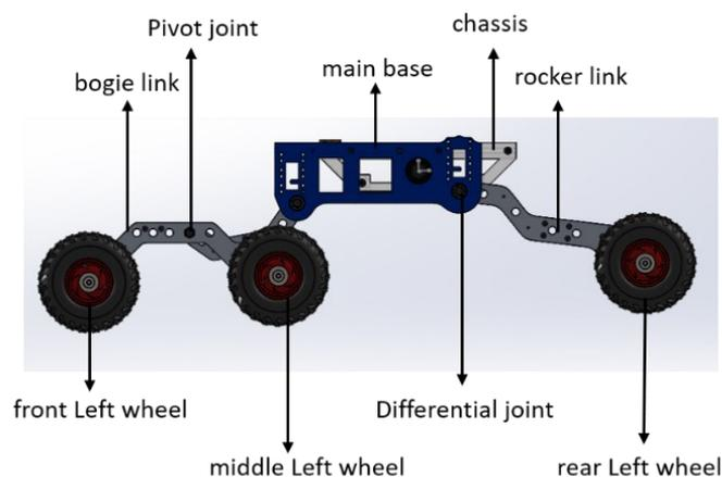
Fig. 1: General view of amphibious robot.
