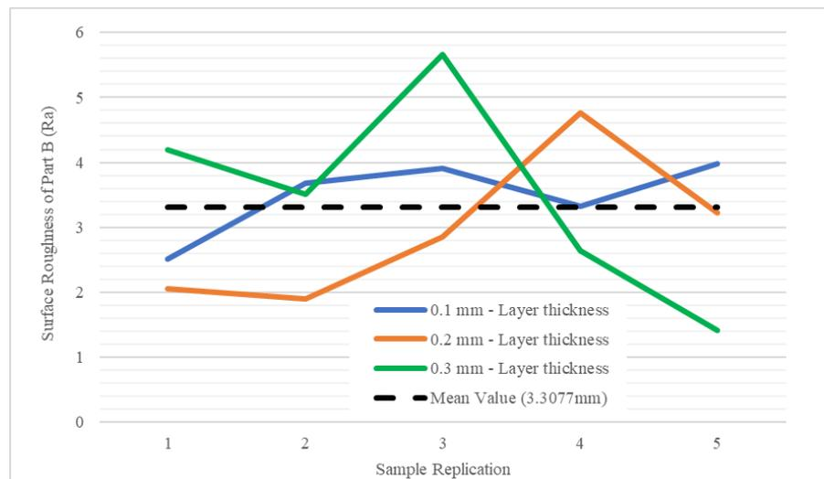
Fig. 4: Trend of surface roughness measurement for Part B.
