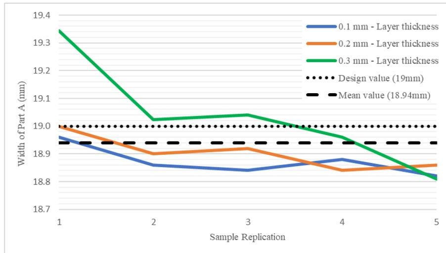
Fig. 3: Trend of width measurement for part A.
