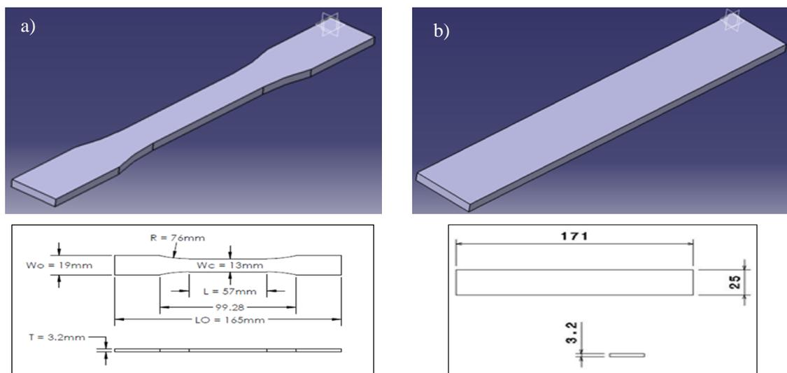
Fig. 1: (a) Part A (above: geometry, below: dimension) and (b) Part B (above: geometry, below: dimension).
