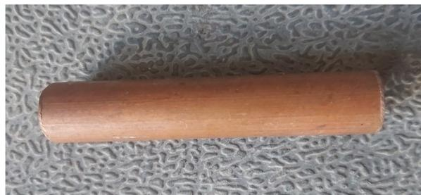
Fig. 2: Copper electrode tool.
