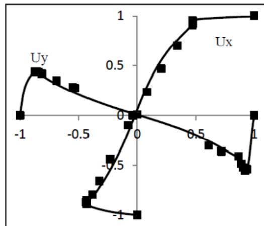
Fig. 1: Velocity profile at mid-height (x-velocity,  $U_x$  and y-velocity,  $U_y$ ) of cavity for  $Re$  number 7500. Line-LBM and symbol- Ghia et al. [3]
