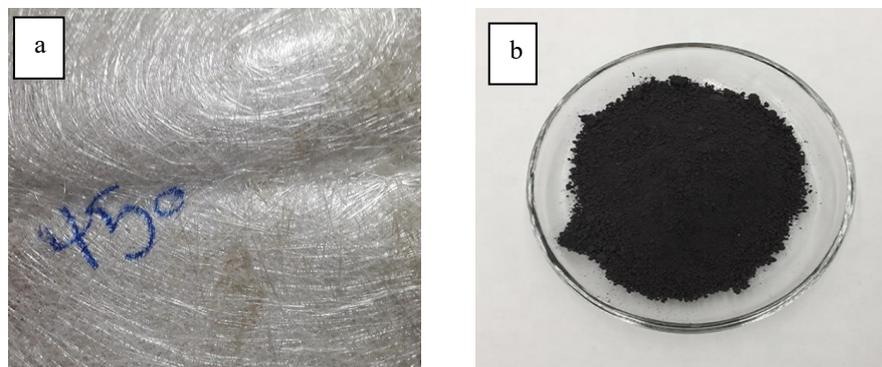
Fig. 1: (a) E-glass fiber chopped strand mat glass fiber, (b) MWCNTs nano-powder.
