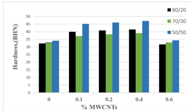
Fig. 9: Comparison between hardness variation and different weight percentages of MWCNTs reinforces polyester/CSM (80/20 wt.%, 70/30 wt.% and 50/50 wt.%).
