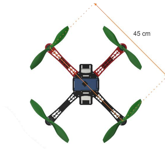
Fig. 9: Mechanics design of quadrotor in top view.
