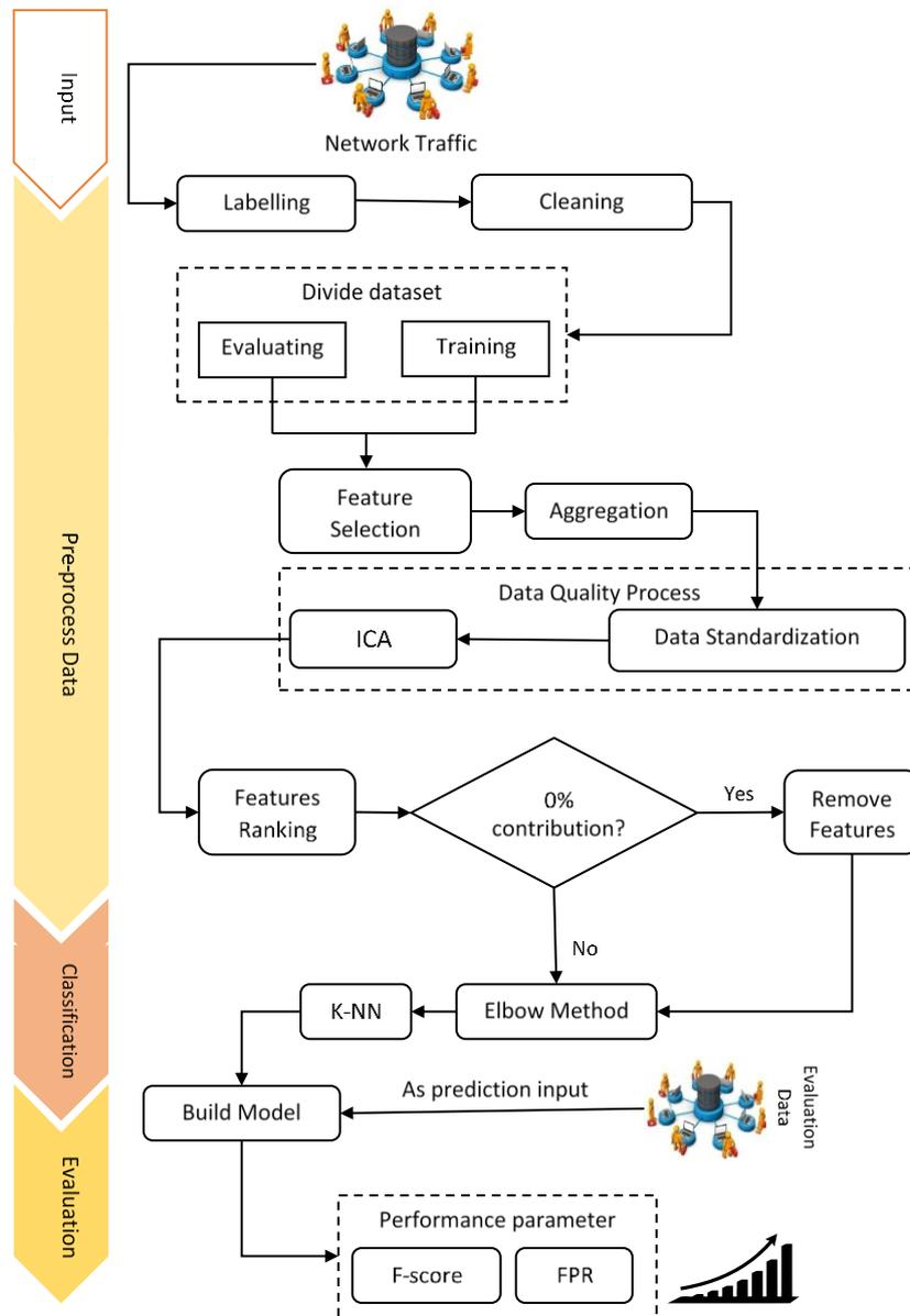
Fig. 2: The proposed framework for pre-processing flow-based features.
