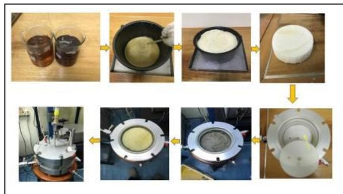
Fig. 2: Procedure of Rowe Cell consolidation test.
