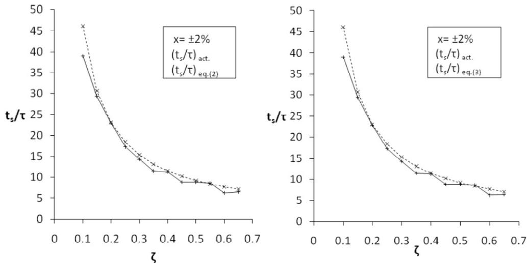
Fig. 2: Actual and calculated  $(t_s/\tau)$  vs.  $\zeta$  for  $\pm 2\%$  settling band.
