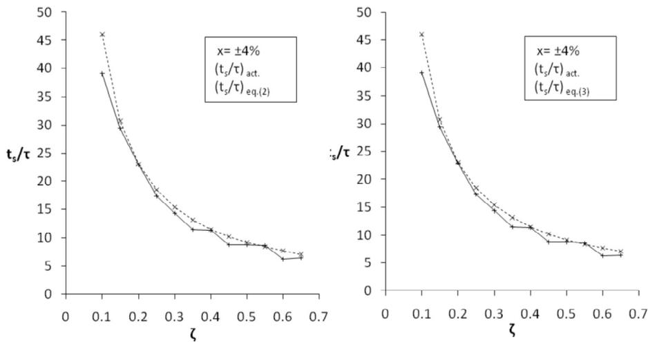
Fig. 4: Actual and calculated  $(t_s/\tau)$  vs.  $\zeta$  for  $\pm 4\%$  settling band.
