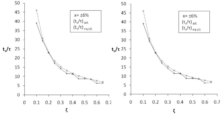
Fig. 6: Actual and calculated  $(t_s/\tau)$  vs.  $\zeta$  for  $\pm 6\%$  settling band.
