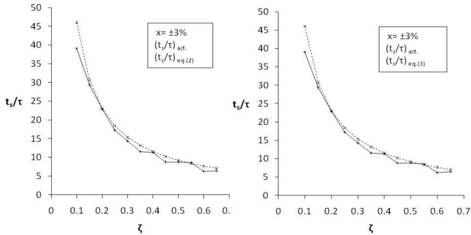
Fig. 3: Actual and calculated  $(t_s/\tau)$  vs.  $\zeta$  for  $\pm 3\%$  settling band.
