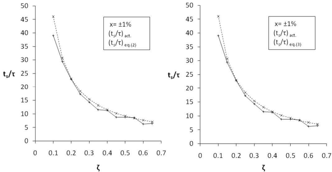
Fig. 1: Actual and calculated  $(t_s/\tau)$  vs.  $\zeta$  for  $\pm 1\%$  settling band.
