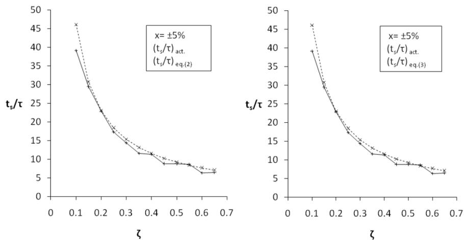
Fig. 5: Actual and calculated  $(t_s/\tau)$  vs.  $\zeta$  for  $\pm 5\%$  settling band.
