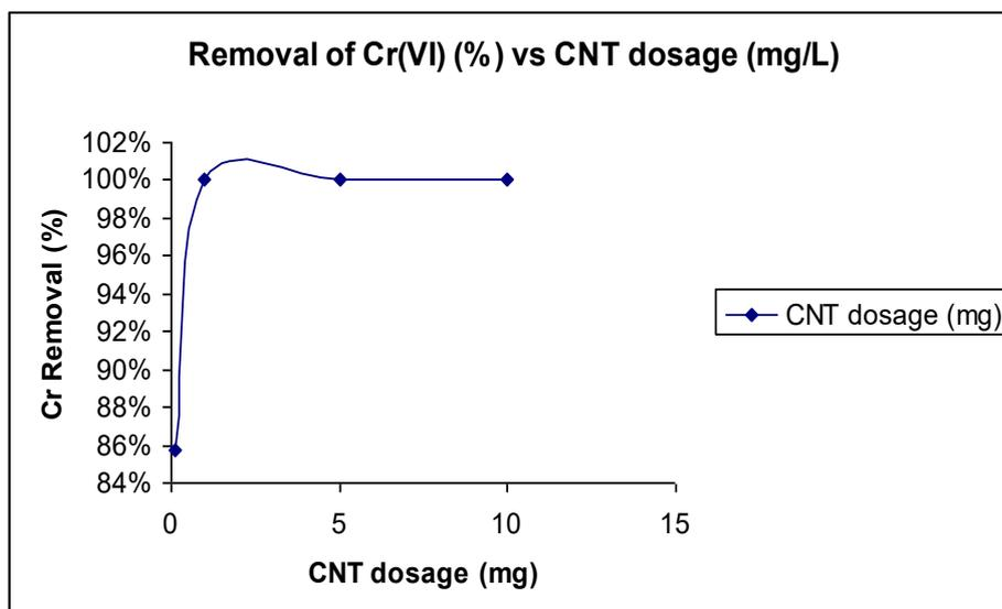
Fig. 2: Impact of CNT amount on Cr(VI) adsorption from solutions at 0.07 mg/L Cr(VI).
