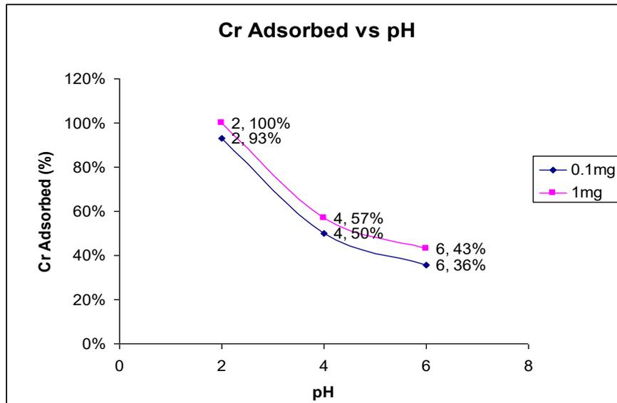
Fig. 1: Impact of pH on the adsorption of Cr(VI) at 0.07 mg/L Cr(VI) concentration.
