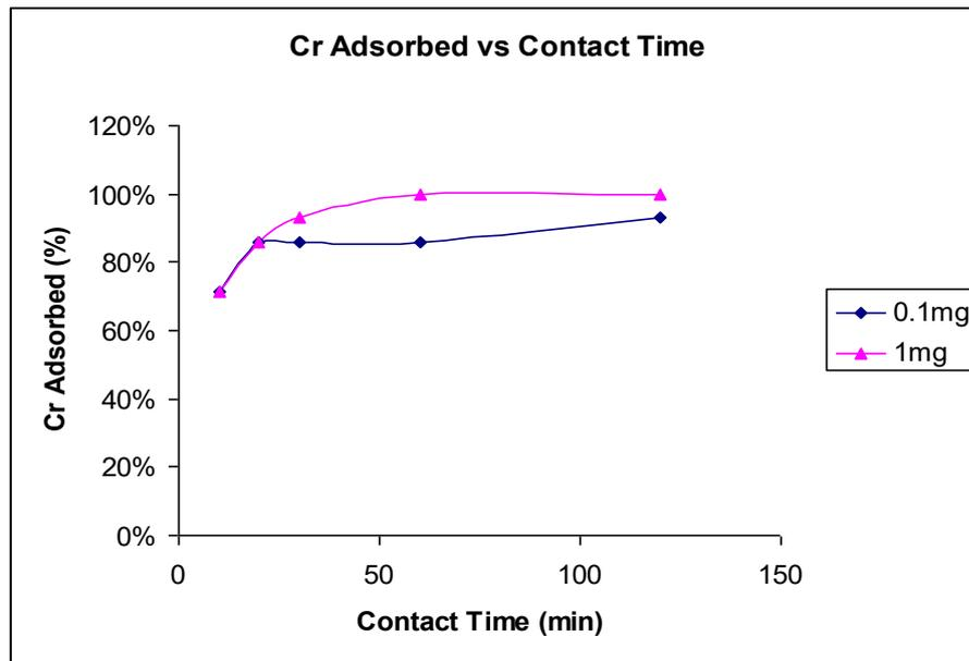
Fig. 4: Impact of contact time on the adsorption of Cr(VI) with [Cr(VI)] = 0.07 mg/L.
