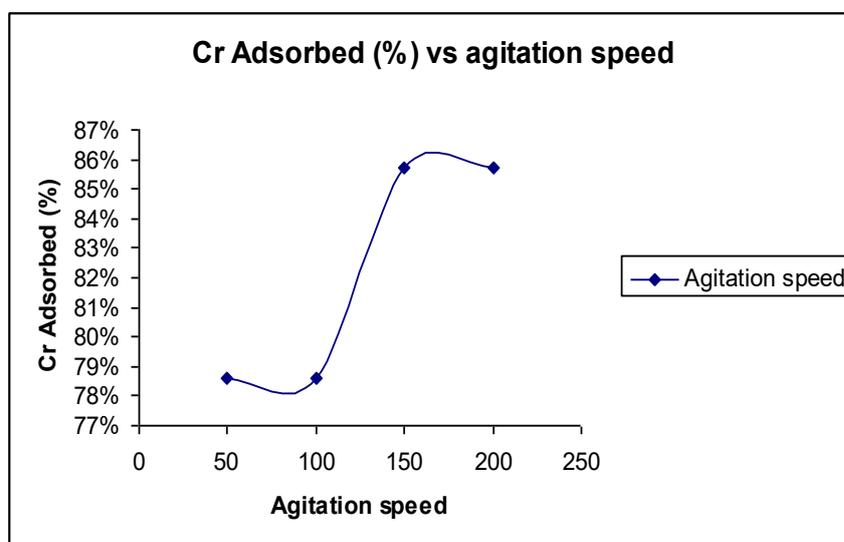
Fig. 3: Impact of agitation speed (rpm) on Cr(VI) adsorption, Cr(VI) concentration=0.1 mg/L.
