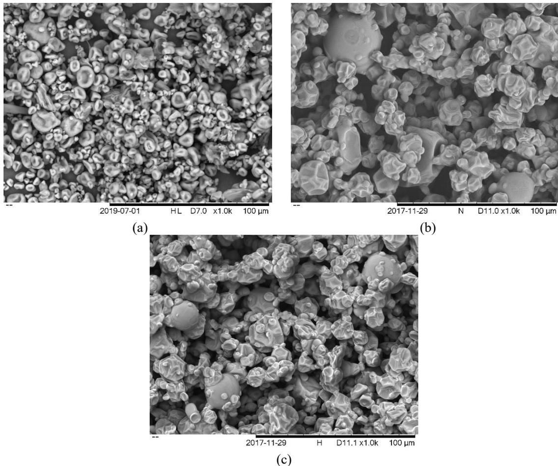
Fig. 4: SEM micrographs of powdered samples obtained at (a) without maltodextrin DE 10 and feed flow rate of 2115 ml/h, (b) with maltodextrin DE 10 and feed flow rate of 2115 ml/h, and (c) with maltodextrin DE 10 and feed flow rate of 485 ml/h. The inlet dry air temperature and air flow rate were fixed at 200 °C and 3.5 m/s, respectively.
