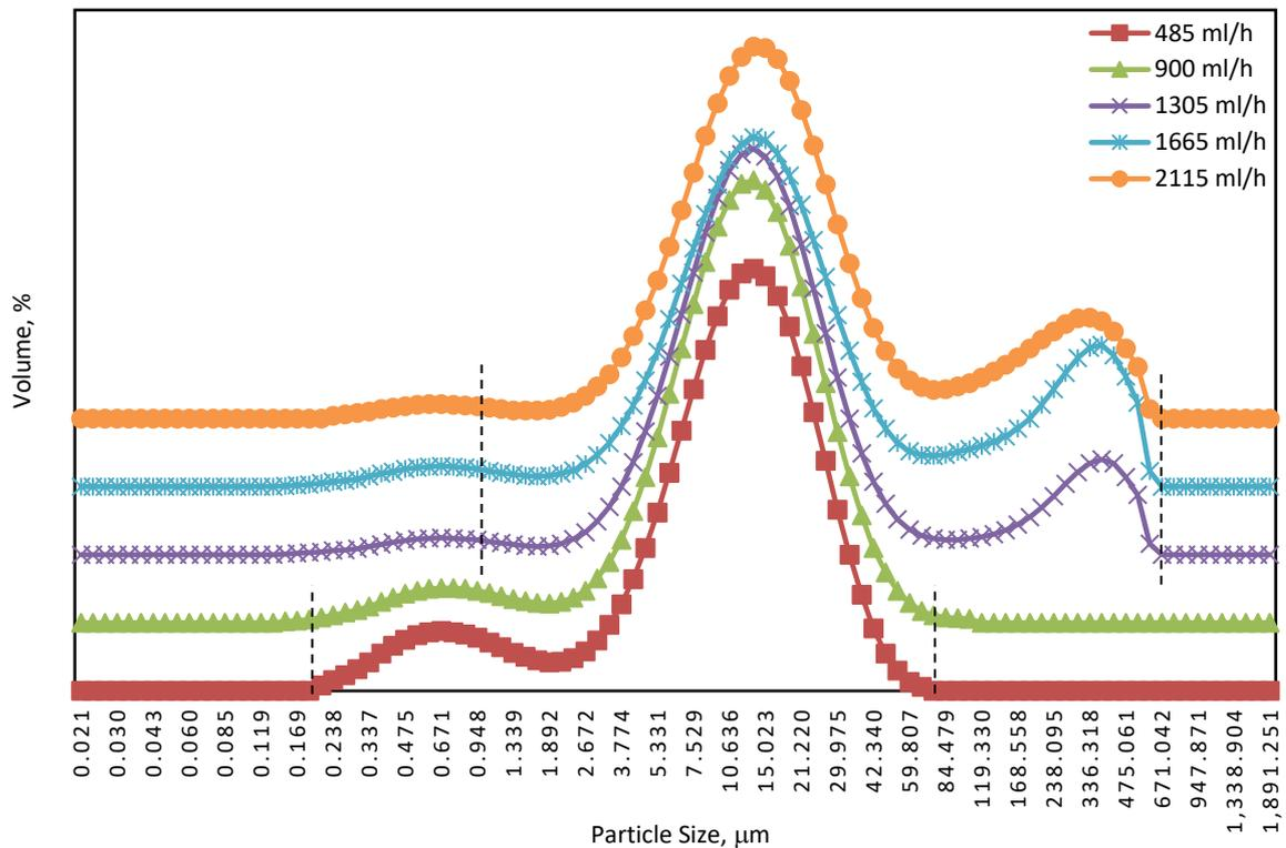
Fig. 3: Particle size distributions of spray dried powder at different feed flow rates.
