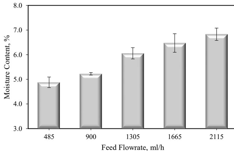
Fig. 1: Moisture content of spray dried powder at different feed flow rates with 0.224 average standard deviation.
