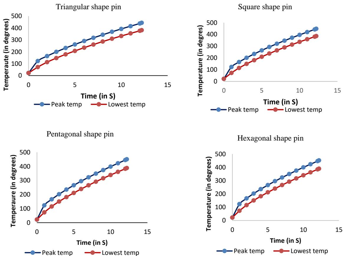
Fig. 8: Transient temperature rises for different pin profiles.
