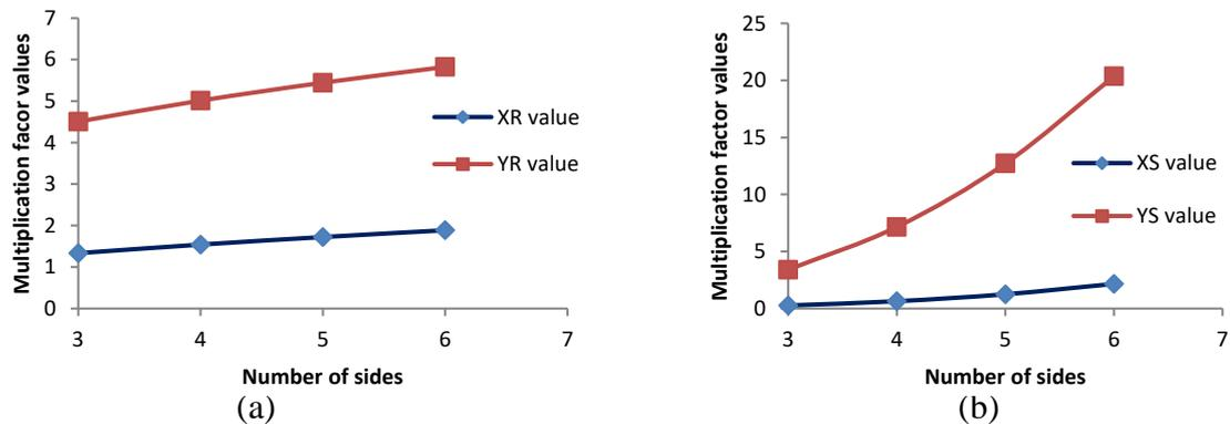
Fig. 6: Change in multiplication values (X<sub>R</sub> and Y<sub>R</sub>) (a) when radius of pin is considered, (b) when pin side length is considered.
