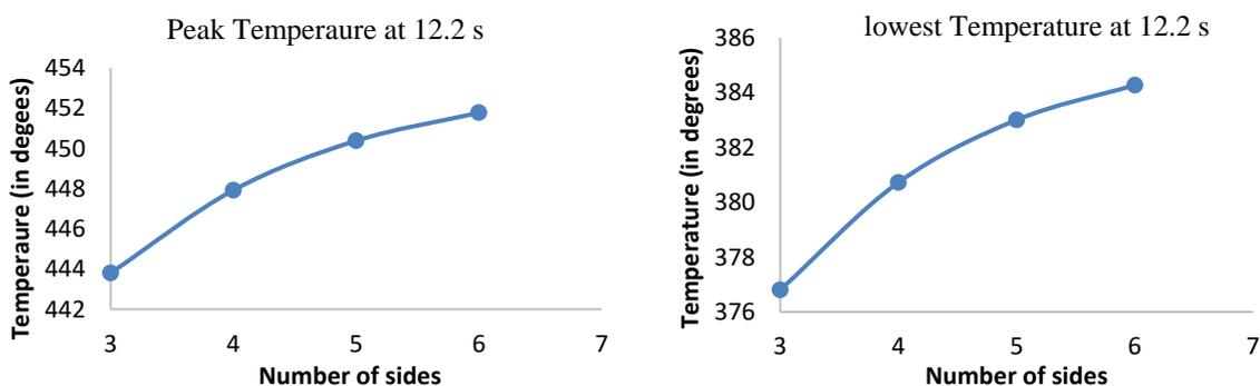
Fig. 9: Change in peak and low temperatures in the stir zone.
