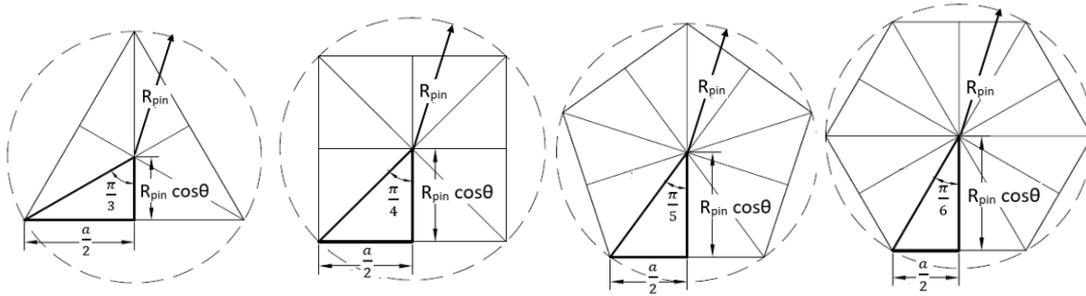
Fig. 4: Cross section of pin profiles and segments.
