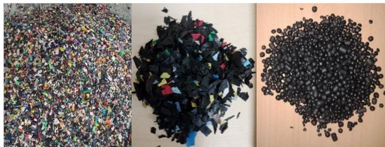
Fig. 4: HIPS Granules and pellets from disposable cups.
