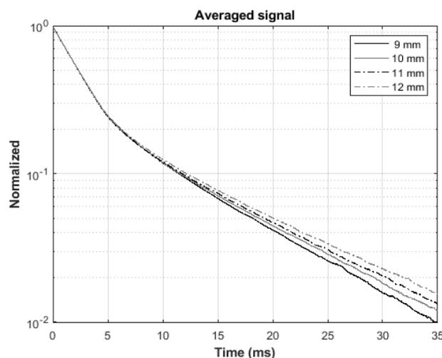
Fig. 5: Typical averaged signals for different sample thicknesses.
