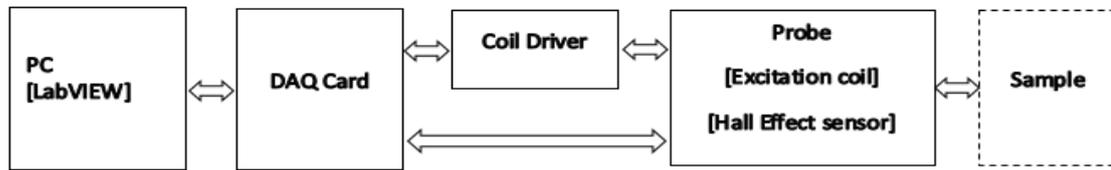
Fig. 4: The block diagram of our PEC system.
