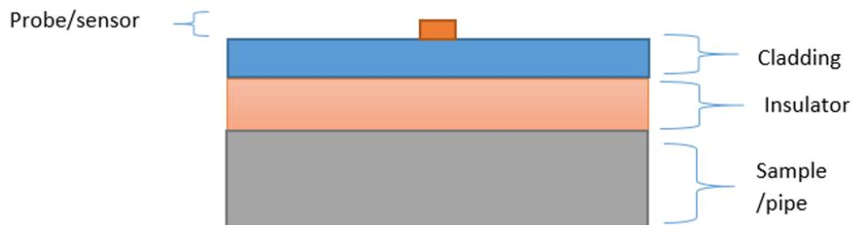
Fig. 1: Typical setting of insulated pipes with a probe sitting on its cladding.
